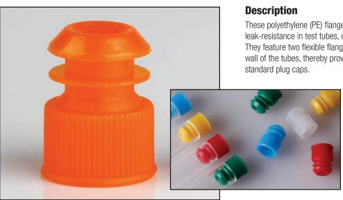
These polyethylene (PE) flanged plug caps provide exceptional leak-resistance in test tubes, centrifuge tubes and round cuvettes. They feature two flexible flanges that press firmly against the inside wall of the tubes, thereby providing better leak-resistance than standard plug caps.
