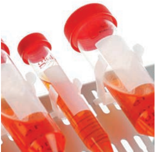
1.5/2.0mL, 15mL and 50mL tube clips are included and can be mixed and matched on the rotisserie tube holder
