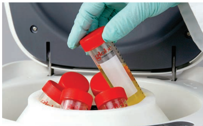
Twelve position rotor compatible with 6 each 15mL or 50mL conical tubes
