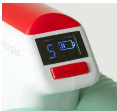
LED display on the Diamond SeroFlow Plus shows the coarse speed setting and battery charge status.
