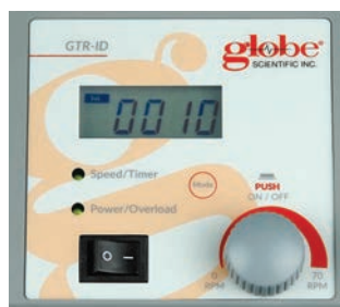
Digital display of the GTR-ID can be accurately set using the parameter adjustment knob
