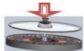
Attach the rotor lid
