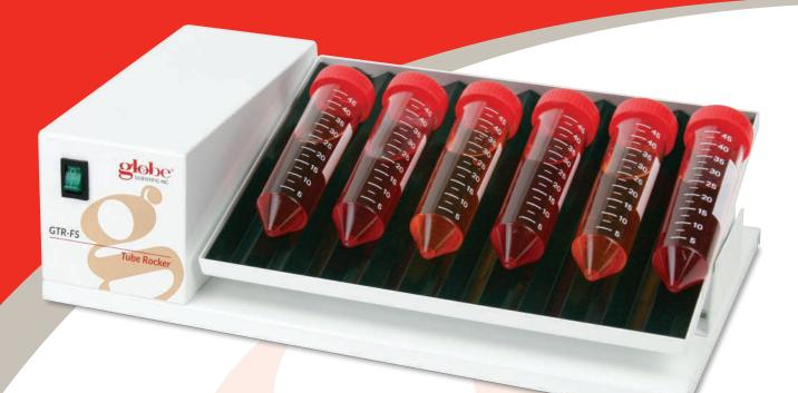
The GTR-FS fixed-speed tube rocker is the best choice for basic laboratory tube mixing applications. With its see-saw motion, a fixed speed of 24rpm and an angle of +/-25° it provides optimal mixing. The ridged platform pad design allows the operator to place any tube from 1.5mL to 50mL on the unit, turn the power switch on and walk away.
