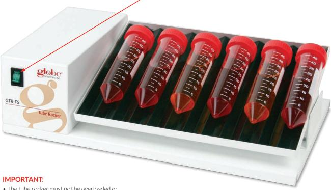
• The tube rocker must not be overloaded or damage may occur. Please do not load the unit in excess of 7lbs (3.2kg).
