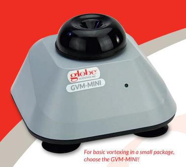
100-240V,50/60Hz Voltage Power 12W Mixing motion Orbital Orbital diameter 4.8mm Motor rating output 10W Speed 3000rpm (fixed) Run type Touch operation Dimensions[WxDxH] 133×133×80mm/5.2 x 5.2 x 3.1in Weight 0.6kg / 1.3lbs Operating Temperature 5 to 40°C Permissible relative humidity 80%RH (non-condensing)
