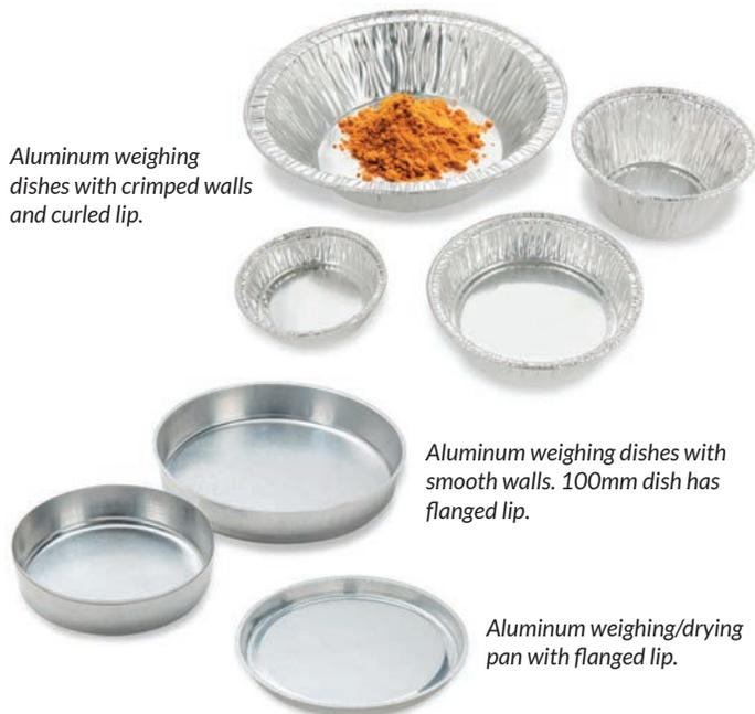
Aluminum weighing dishes with crimped walls and curled lip.
